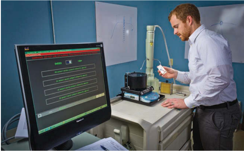
Engineer Chris Cummings inspects an acrylic block that was ablated in a test using a water-filled verification unit.
